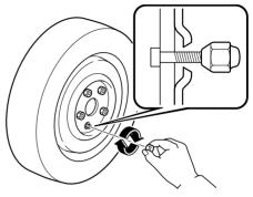
Do not apply oil or grease to lug nuts and bolts and do not tighten the lug nuts beyond the recommended tightening torque:
